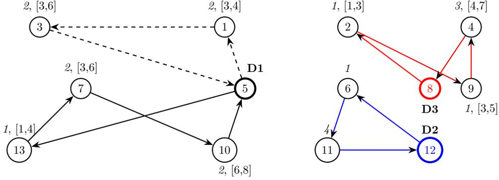
Figure 2: A Small Example of a Multi-depot Capacitated Vehicle Routing Problem with Time Windows (MDCVRP-TW)
