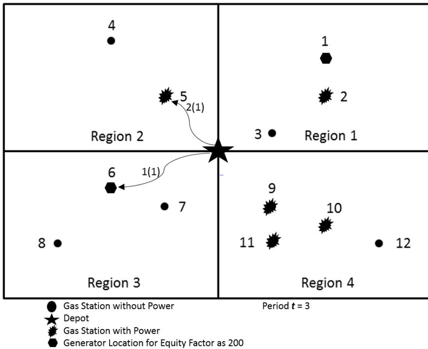
Figure 7: Truck Assignments for Scenario 3 Period 3.
