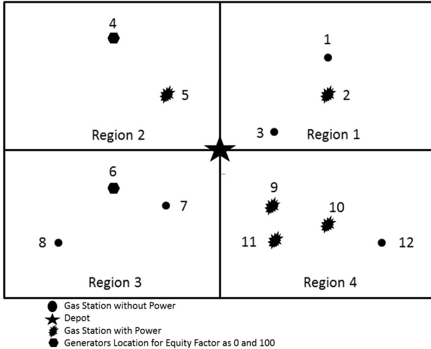
Figure 3: Generator Placement for the Illustrative Example.
